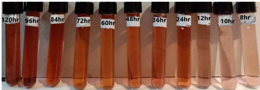
Fig. 3. Biosynthesis of ULAgNPs kept at different incubation time intervals at static conditions at 30°C.
