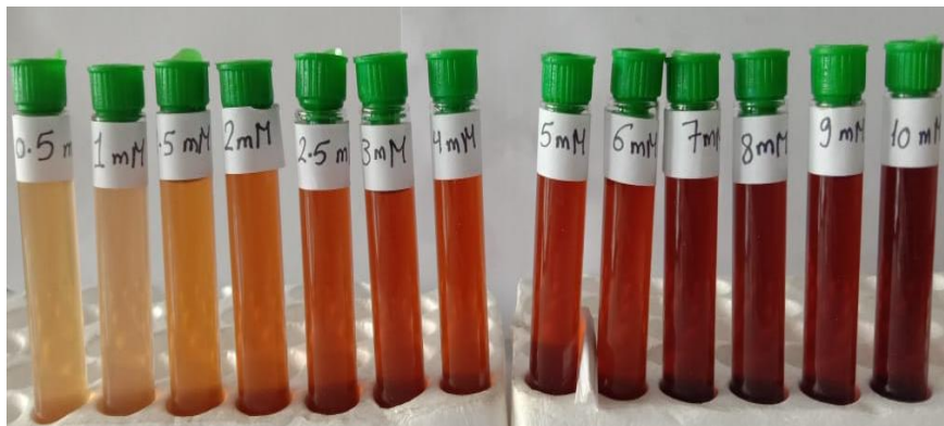
Fig. 7. Effect of different concentrations of AgNO 3 (in mM) on ULAgNPs biosynthesis containing 5:5, v/v ratio at static conditions and 30 °C for 48 hr.
