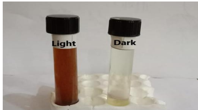
Fig. 11. Biosynthesis of ULAGNPs in reaction solution containing (5:5, v/v) ratio of 4mM AgNO 3 kept at static condition for 84h in dark and light conditions.
